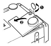
4. Use a screwdriver, coin, or similar object to loosen the two screws holding the lamp in position. *(You* cannot remove these screws.)
