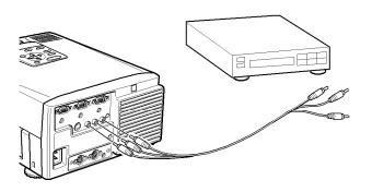
4. Connect the other plugs on the audio/visual cable to the Audio In jacks of the projector: insert the white plug into the L Audio In jack and the red plug into the R Audio In jack. Connect the plug at the other end of the audio/visual cable to the audio output jacks of the video source.
