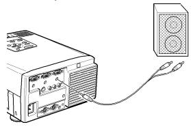
3. Connect the RCA plugs to the external amplified speaker or PA system. Insert the cable's red plug into the Audio In R jack, and the white plug into the Audio In L jack.
